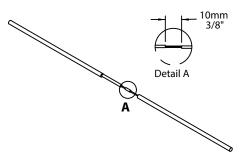
2.8 Insert the 4 x 40 heat shrink tube over the connection and make sure it is centered to the mechanical connection. Then heat the entire length of the tube with a hot air gun (do not overheat it), make sure the tube has shrunk enough to see the sealant coming out of both sides.
