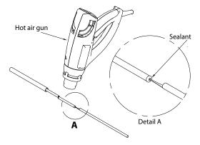
2.6 Insert the 4 x 40 heat shrink tube into one of the 60 mm (2 3/8") cut wires.
