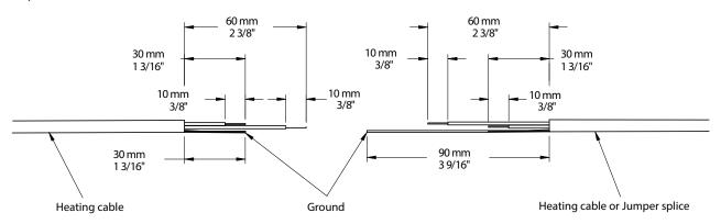
$2.3 \quad \text{Cut the 6} \times 80 \text{ to 65} \text{ mm } (2\,1/2") \text{ long heat shrink tube and insert } \text{ into the earlier ground cut at } 90 \text{ mm } (3\,9/16").$
