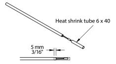
5.4 Heat the entire length of the heat shrink tube with a hot air gun (do not overheat it), make sure the tube has shrunk enough to see the sealant coming out of both sides.
